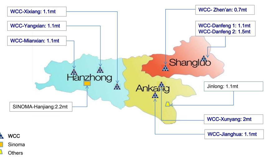
Indicated tonnage is annual cement capacity. Source: Digital Cement, WCC
